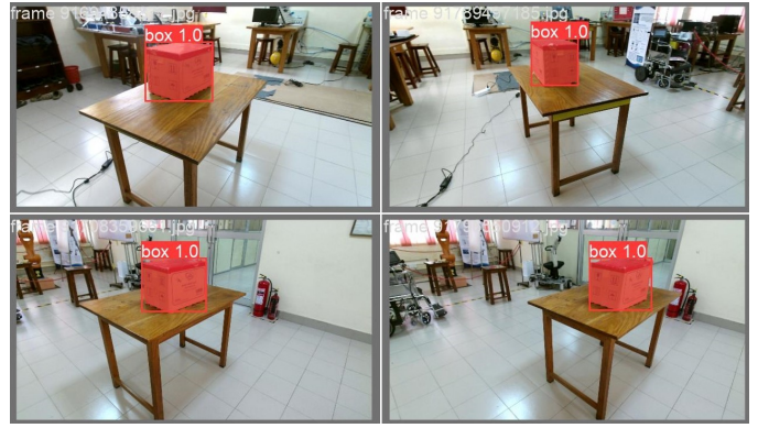
Fig. 3. Segmenting a box-shaped object to isolate it from the background
