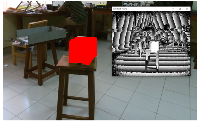
Fig. 6. Difference between the image frame and the depth frame after masking the object
