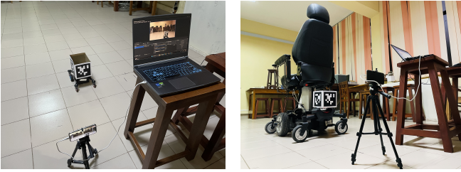
(a) Localization System of CasteriX (b) Localization System of Jazzy Air Fig. 3. Localization Systems of both robots
